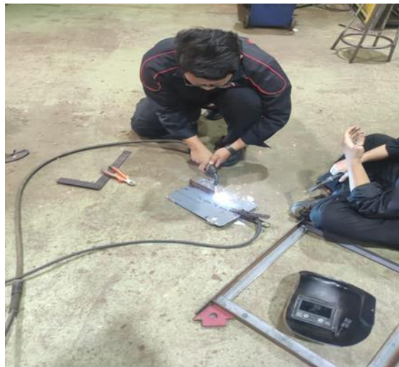
Rajah 3.3.2.5 Proses kimpalan plat dijalankan.
