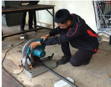
Rajah 3.6 proses memotong besi
