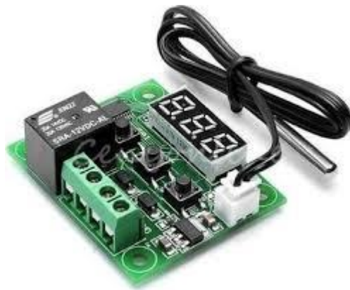
RAJAH 2.8 Temperature Sensor Control Switch Thermostats
