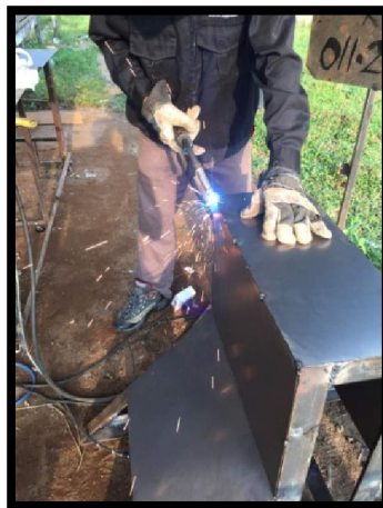
Rajah 3.22 : Mengimpal plat besi ( mild steel )
