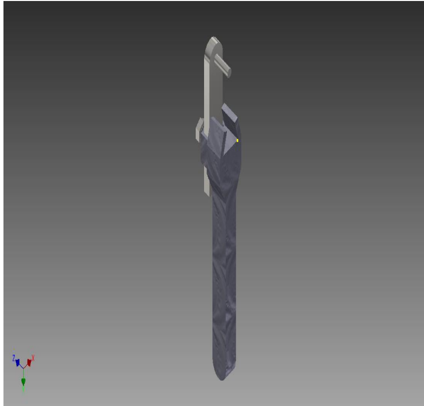
Rajah 3.7 : Lukisan Inventor Alat Penegang Rantai Motosikal
